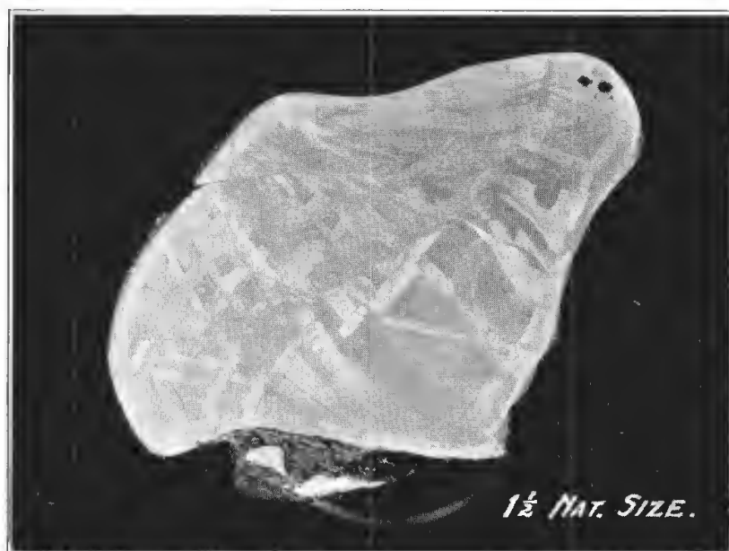
Fig. 7. Etched section of the iron showing the wavy nature of the kamacite bands. Several long, closed cracks may also be seen.
